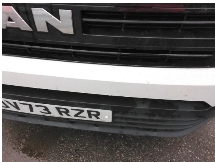
1: Panel Front Chipped Multiple Chips
