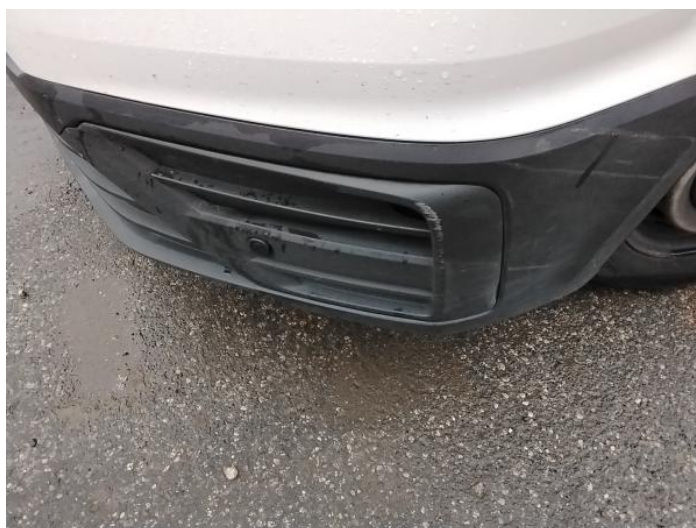
2: Bumper Front Moulding Scuffed (Unpainted) Over 100mm
