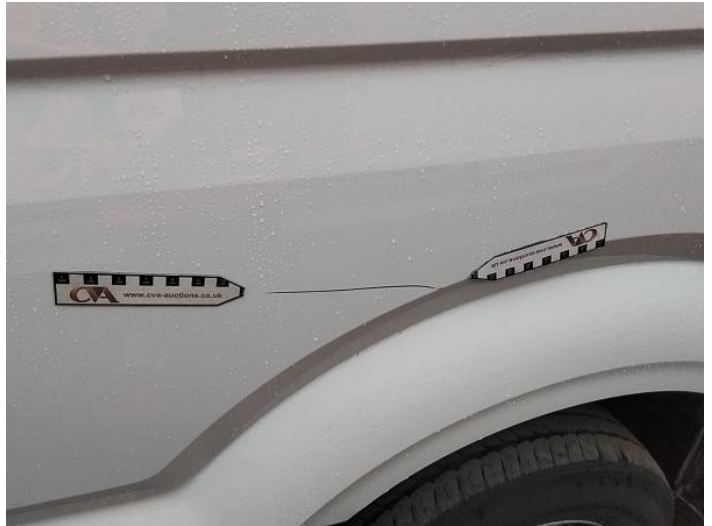
4: Qtr Panel osr Scratched Over 25mm Thru Paint
