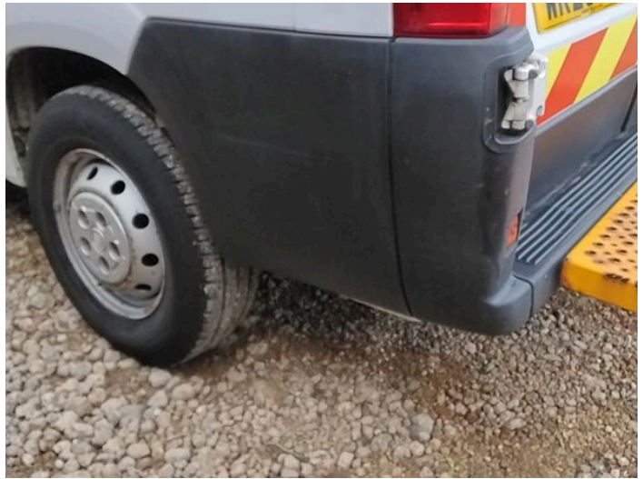
6: Bumper Rear Moulding Scuffed (Unpainted) UpTo 100mm
