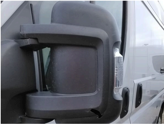
5: Door Mirror Assy nsf Broken Replace
