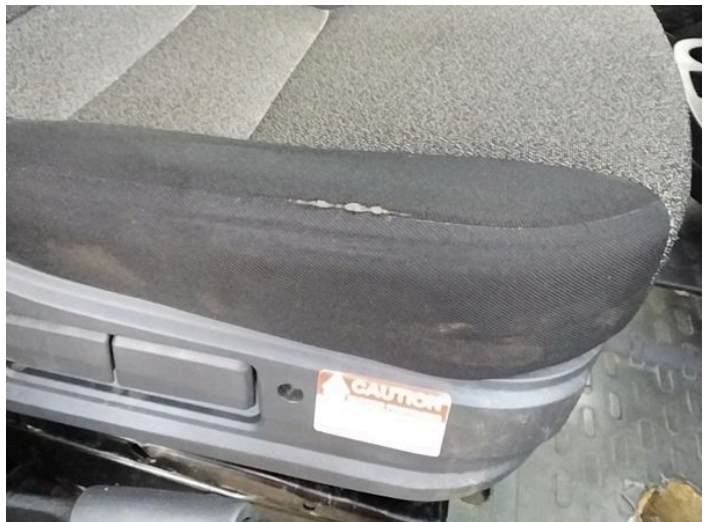
8: Seat Base Cover osf Holed Over 3mm
