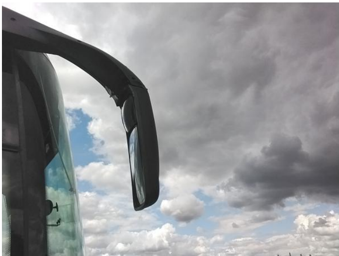
15: Door Mirror Assy osf Broken Replace
