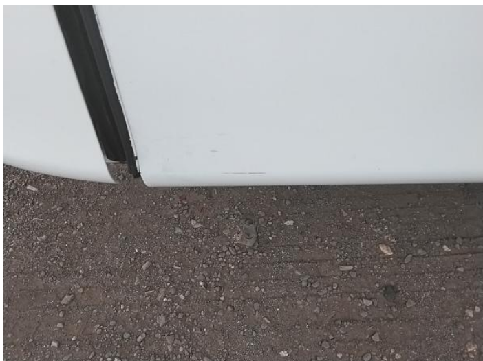
3: Door nsf Scratched Over 25mm Thru Paint
