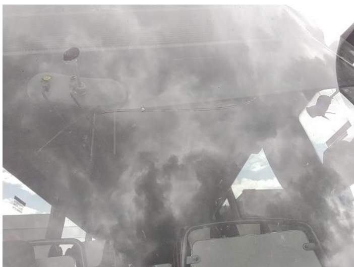
1: Screen Front Cracked Replace
