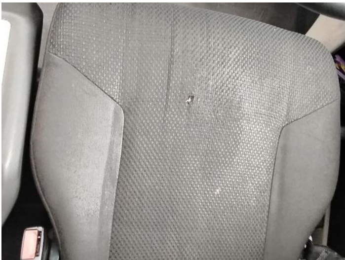
16: Seat Base Cover osf Holed Over 3mm
