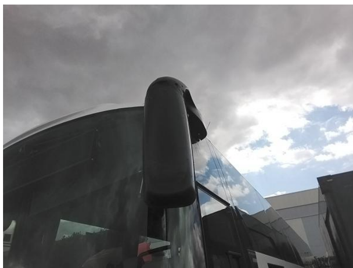
2: Door Mirror Assy nsf Broken Replace
