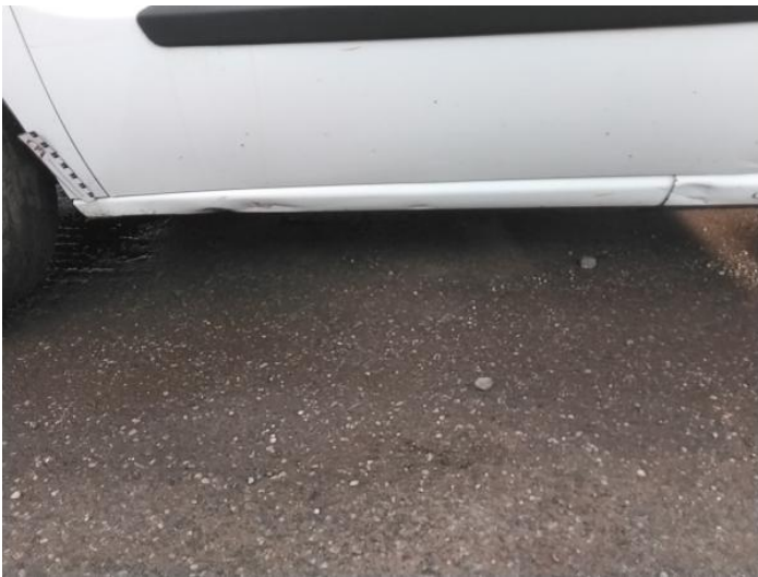
5: Sill ns Dented Over 30% Of Panel
