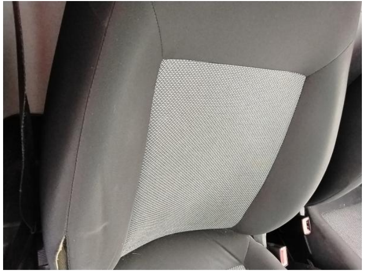
16: Seat Back Cover osf Torn Over 3mm
