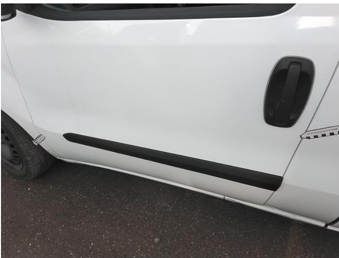
7: Door nsf Scratched Over 25mm Thru Paint
