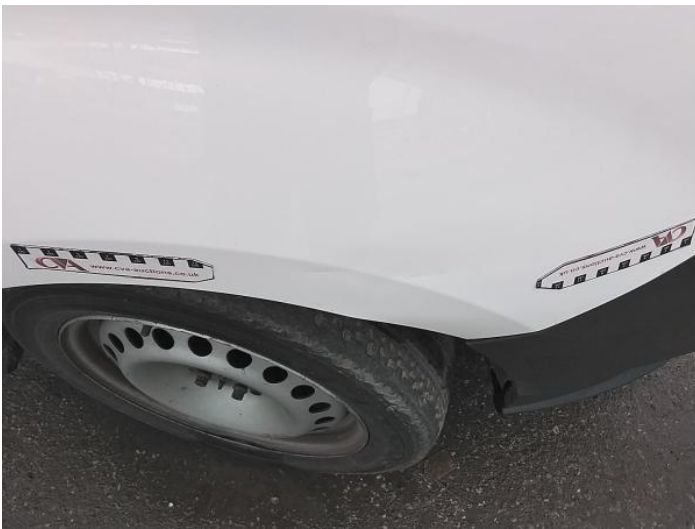
11: Wing osf Dented With Paint Damage
