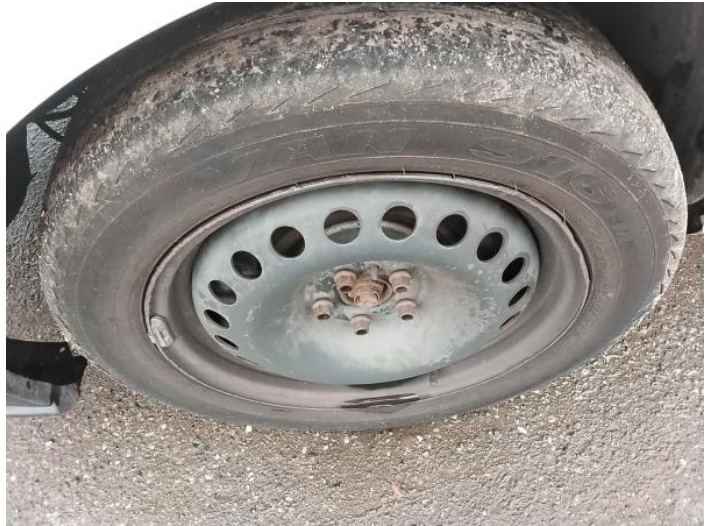
4: Wheel nsf Dented Over 30mm (Steel)
