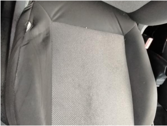
15: Seat Base Cover osf Torn Over 3mm
