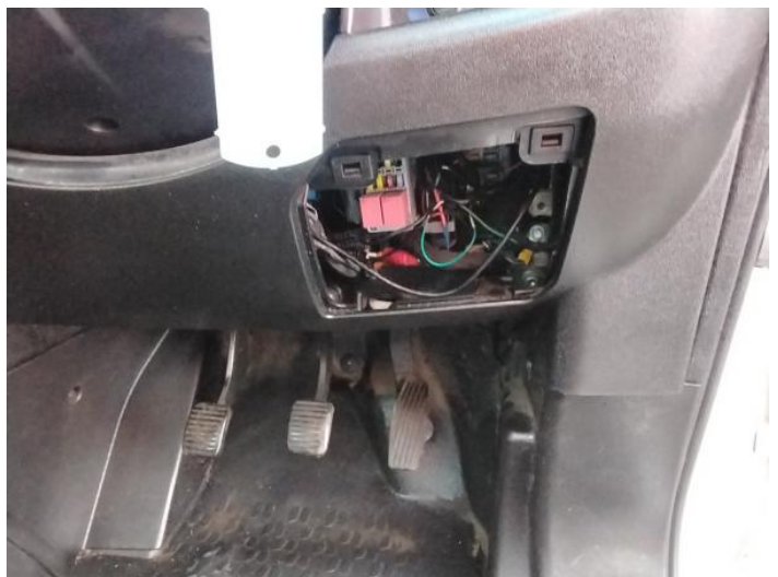
14: Fascia Panel Missing Replace
