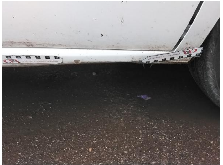
10: Sill os Dented With Paint Damage
