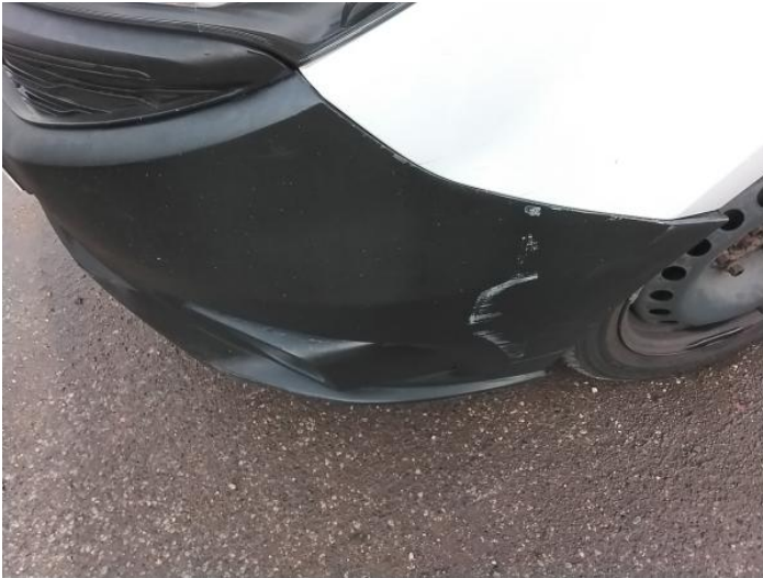
3: Bumper Front Scratched Over 100mm Thru Paint
