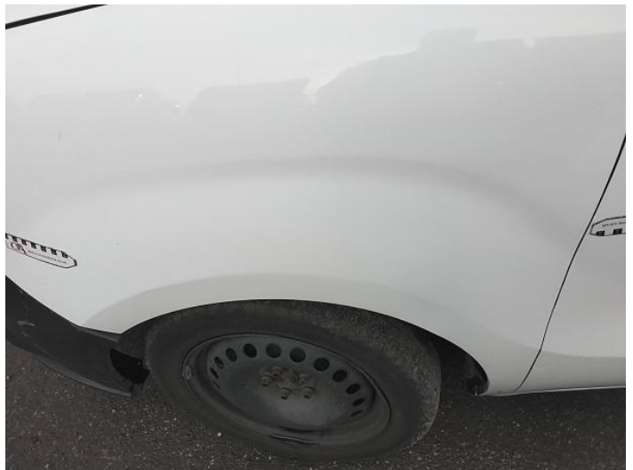
6: Wing nsf Scratched Over 25mm Thru Paint
