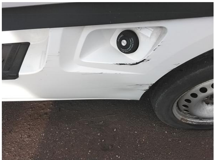
8: Qtr Panel nsr Dented With Paint Damage
