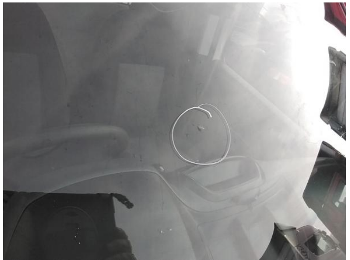
12: Screen Front Chipped Over 10mm
