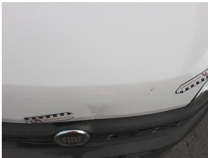
2: Bonnet Dented With Paint Damage
